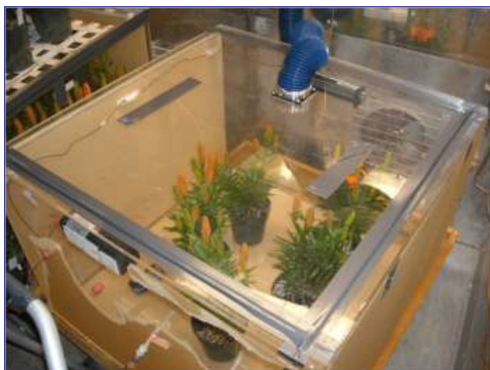
Figure 1. Chamber (here with lily plants) in which bulbs were treated with ethylene. The air stream containing 10 ppm ethylene entered via the fitting on the front, and was exhausted through the blue tube attached to the top of the chamber.
